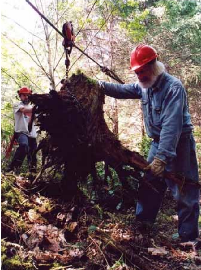
Figure 14. With the skyline raised, Ken Millard guides a stump out of the windrow while Odin Scholz lets out line on the block-and-tackle. (Photo by Brian Mitchell)
