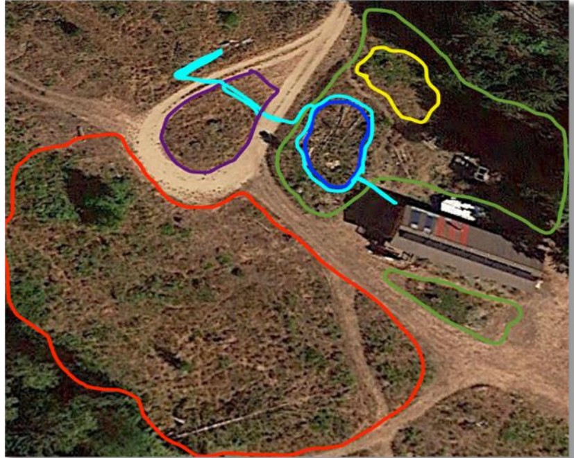
Figure 12: The flowpath of water as it moves through the system. Right to left from this perspective: off of the roof, through the primary swale, into the wetland, through the first culvert, through the secondary swale, through the second culvert
