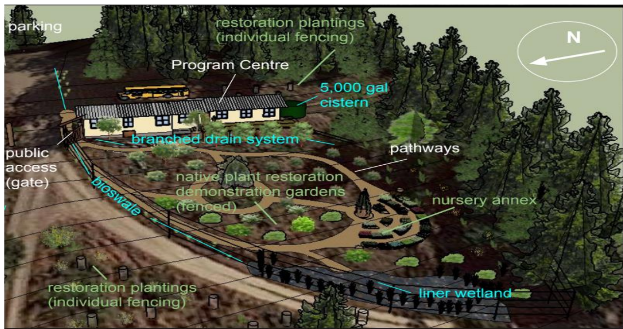
Figure 5: Illustrated schematic of the Program Centre project. This included the construction of the building itself, as well as the restoration of the areas around it with demonstration gardens, a nursery annex, a bioswale, and liner wetland. Photo: GCA
