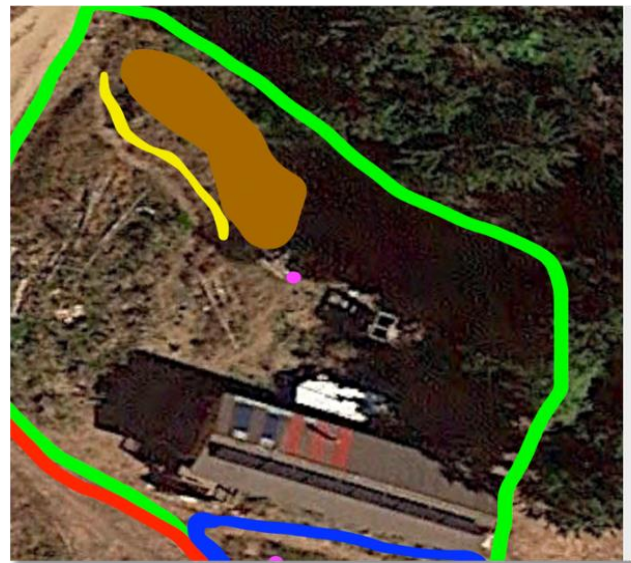
Figure 8: Green polygon, the brown area represents the septic leach field, and the yellow line indicates the location of the buried powerline
