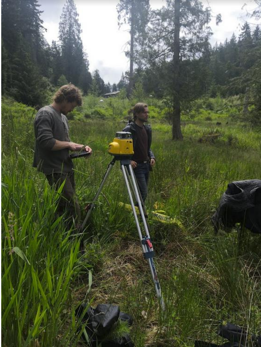
Figure 1: Fin and Karlis near the laser level during the slope survey on the potential wetland site. Photo: Coline Laurent.
