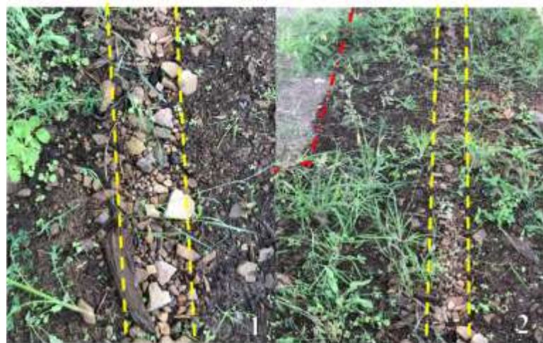
Figure 2B. Photograph of conditions underneath the first array. Image 1 shows a close view of the erosion line caused by the solar array runoff. Image 2 shows the erosion line, as well as the evident separation between the parts of the plot which receive run-off, and the parts of the plot which do not receive any run-off water. The yellow dashed line outlines the erosion line which runs through the centre of the plot. The red dashed line outlines the dry zone which does not receive any run-off rainwater.
