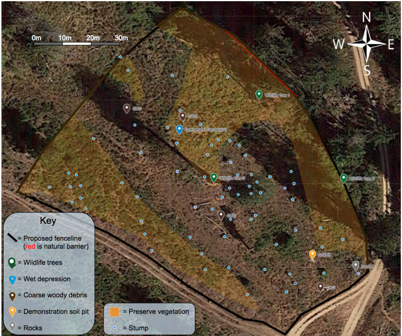
Figure 8: Guide for restoration prescription, showing proposed fenceline, areas of vegetation and stumps to preserve during machine work, coarse woody debris piles to redistribute, and significant features to retain.
