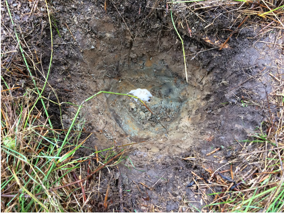
Figure 42: Soil pit for Quadrat 3, showing increasing dominance of finer sediments, gleying, and water table.
