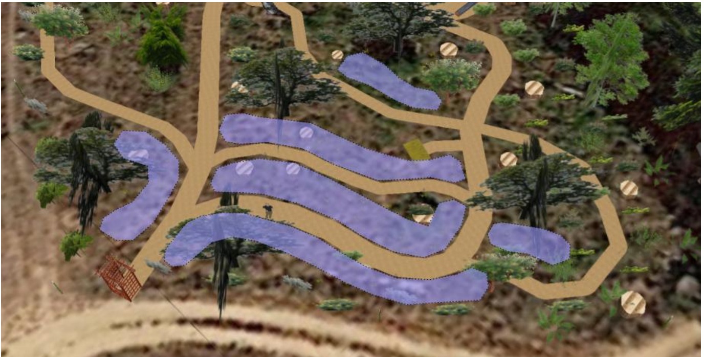
Figure 54: Proposed locations of Garry oak Meadow Garden swale berms, with pathways serving as depressions. Relative proportions and positions will shift based on spatial considerations and contour. Swales can be established over time as desired, depending on the success of the initial plantings. Stumps can be removed or incorporated into berms.
