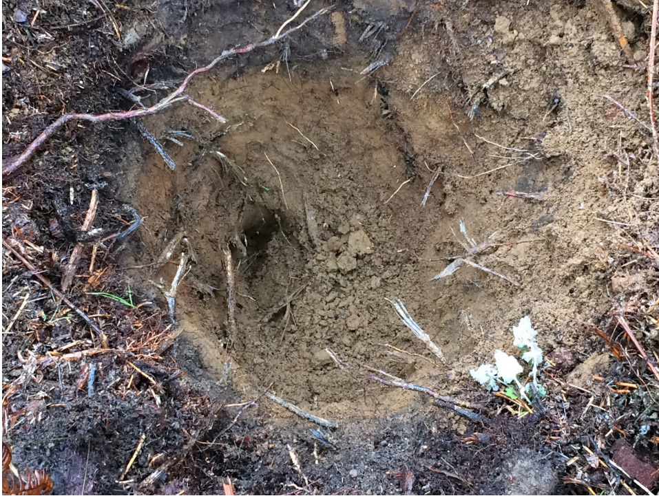
Figure 40: Soil pit for Quadrat 2, showing enriched Ah horizon, loamy sand B horizon, and charcoal layer.
