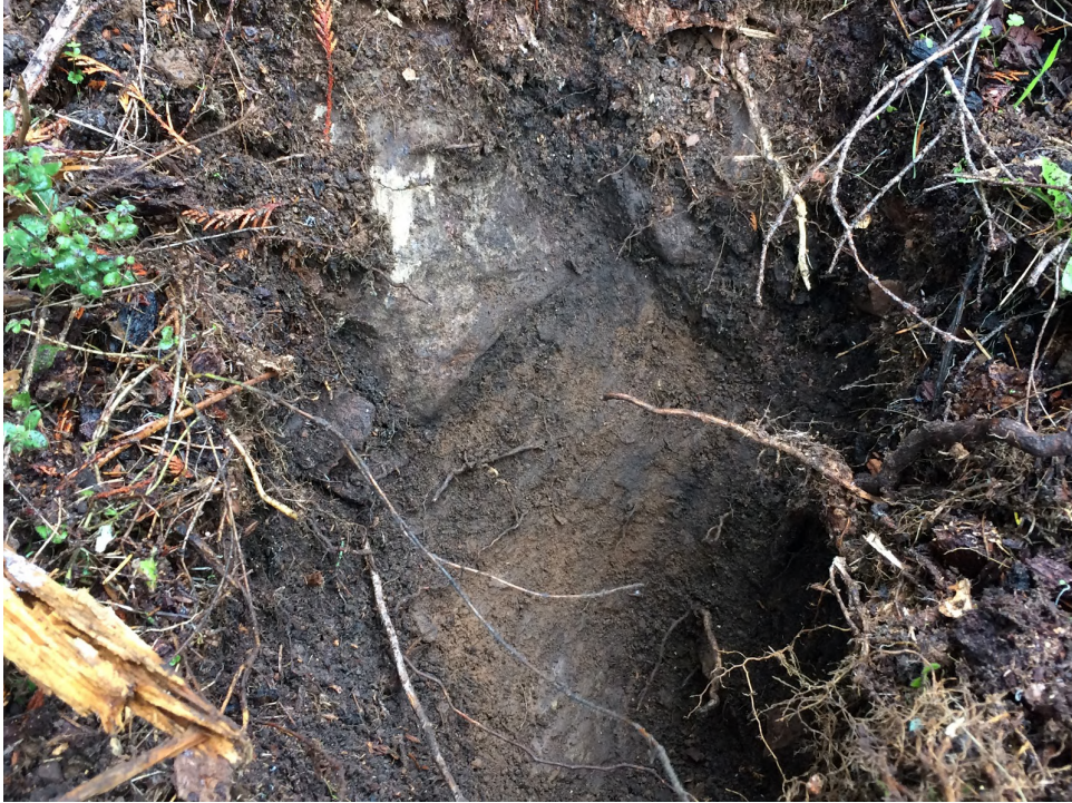
Figure 52: Soil pit for Quadrat 8, showing enriched LFH and Ah horizons, high coarse fragment content, and sandstone bedrock at 50 cm.
