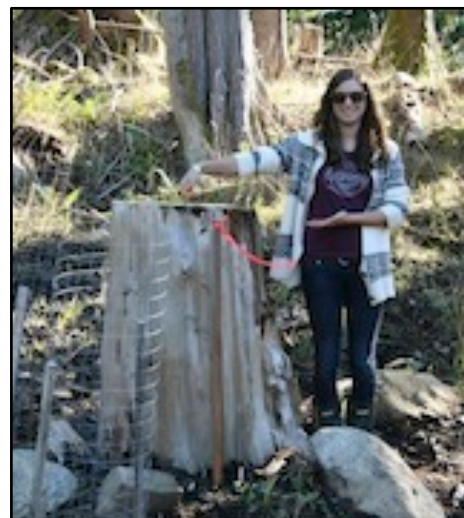
Figure 4. The benchmark of the Y-axis is the pith of this stump
