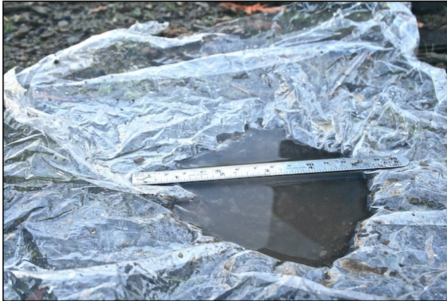
Figure 6. Measuring bulk density using the soil excavation and water replacement method. I used a ruler to ensure that the cavity was completely filled with water. Photo taken on October 29 th , 2014
