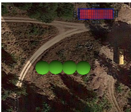
Figure 2.4-1 Shade losses of a north-south tree canopy (4 individuals of 3.6m radius) 10 meters from reference rock at 5-35m heights
