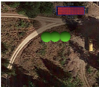
Figure 2.4-1 Shade losses of a north-south tree canopy (4 individuals of 3.6m radius) 10 meters from reference rock at 5-35m heights
