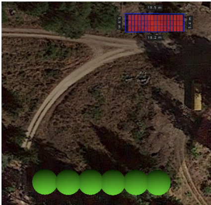
Figure 2.4-4 Shade losses of a north-south tree canopy (6 individuals of 4m radius) 40 meters from reference rock at 5-75m heights
