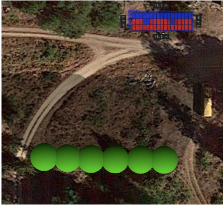
Figure 2.4-3 Shade losses of a north-south tree canopy (6 individuals of 4m radius) 30 meters from reference rock at 5-75m heights
