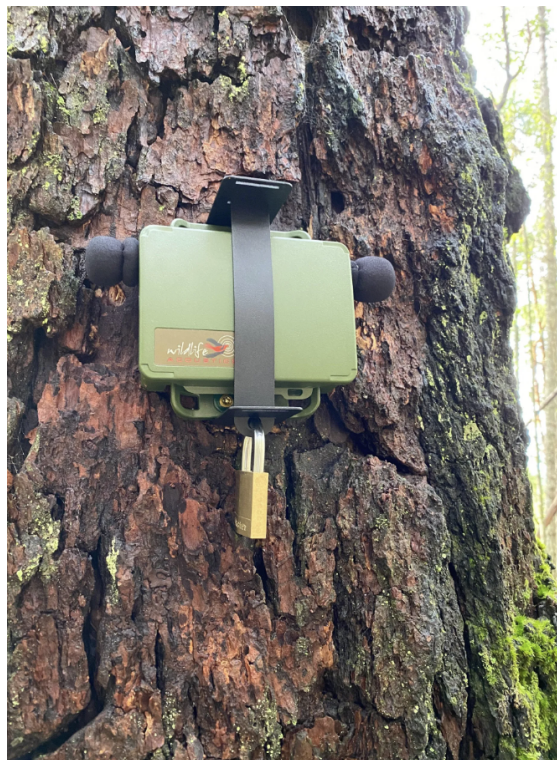
Figure 1. A passive acoustic monitoring audio device, fixed to a Douglas fir tree. Photo credit: Ren Ferguson (2022)
