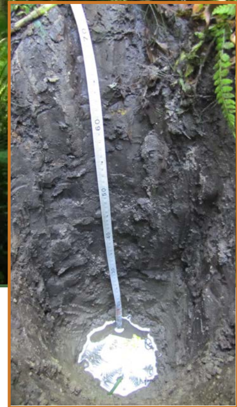
Soil Pit 11 SMR: 7f SNR: R-VR Organic Layer: 35 cm Soil Texture: Clay, Sand
