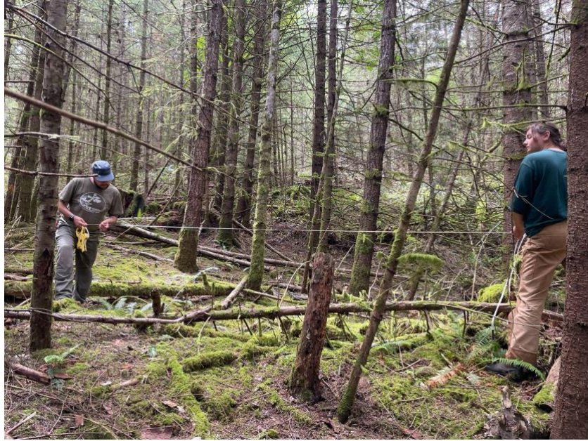
Figure 4: Photo showing the process of measuring the length of CWD using a 30-metre open reel tape measure. Ruth (right) holds the end of the tape at one end while Kyle (left) reads the length at the other end. Both ensure that the places they hold the tape align with the start and end of the section of the log whose diameter is at or greater than 7.5 cm.
