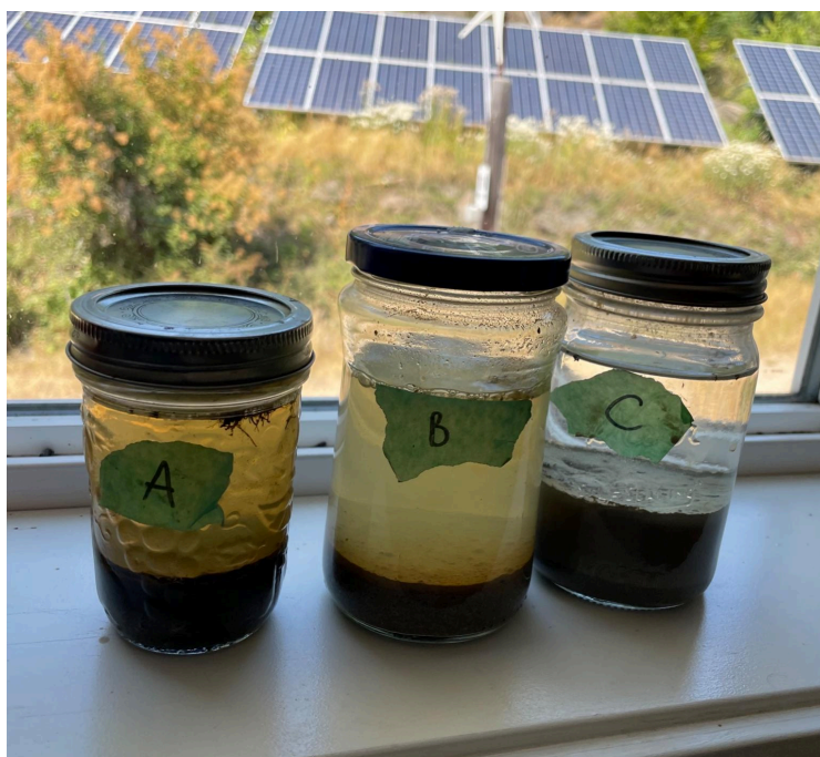
Figure 11. Soil horizon jar test conducted by GCA staff on July 5th, 2024. [A layer = loam (53% sand, 36% silt, 11% clay). B layer = sandy loam (80% sand, 5% silt, 15% clay). C layer = clay (24% sand, 76% clay) (Huggins, 2024)]
