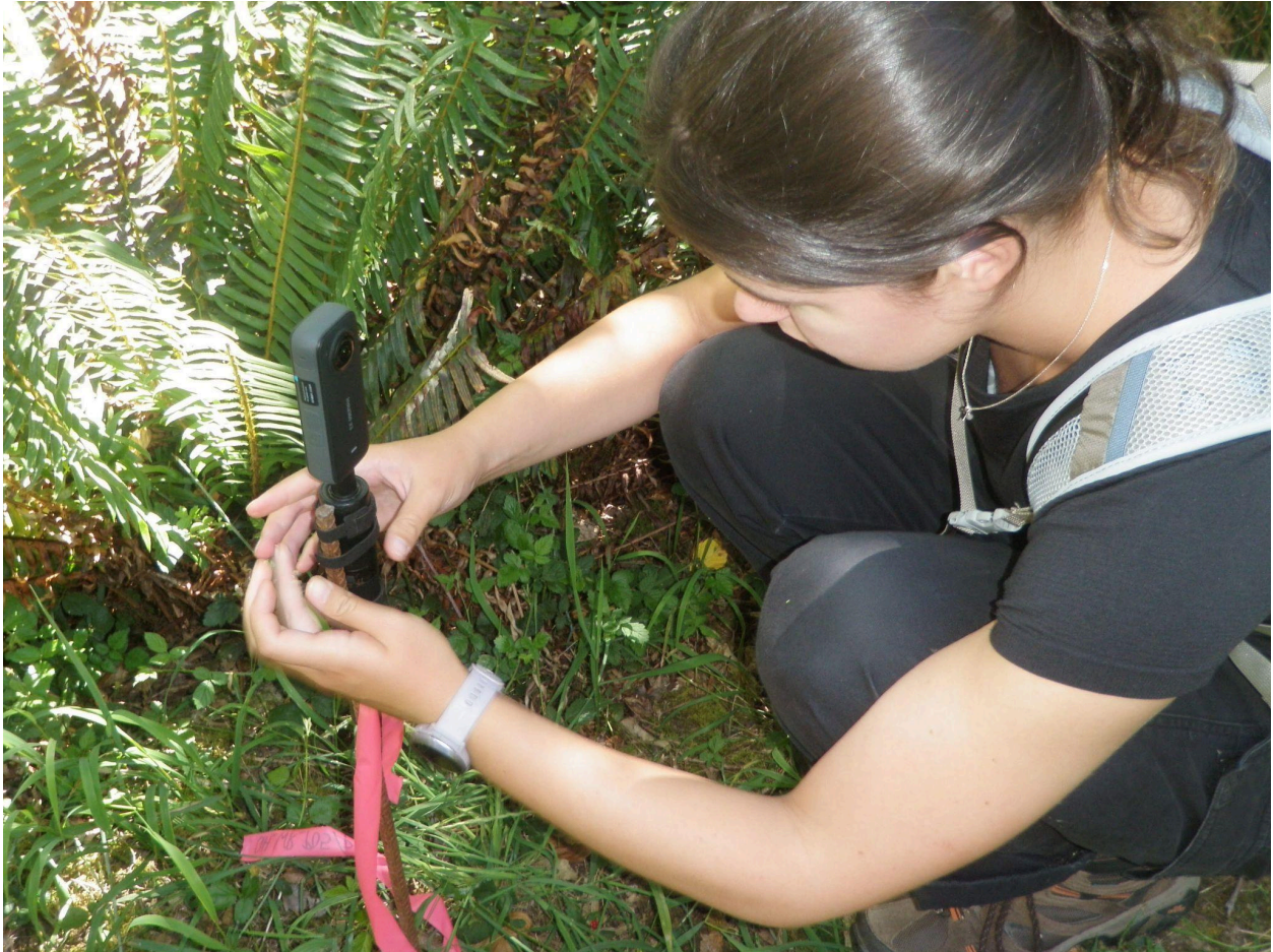
Figure 7: Insta360 camera being strapped to a rebar stake. In this image the camera has yet to be unfolded into its full height. Image credit: Chelsea Deren.
