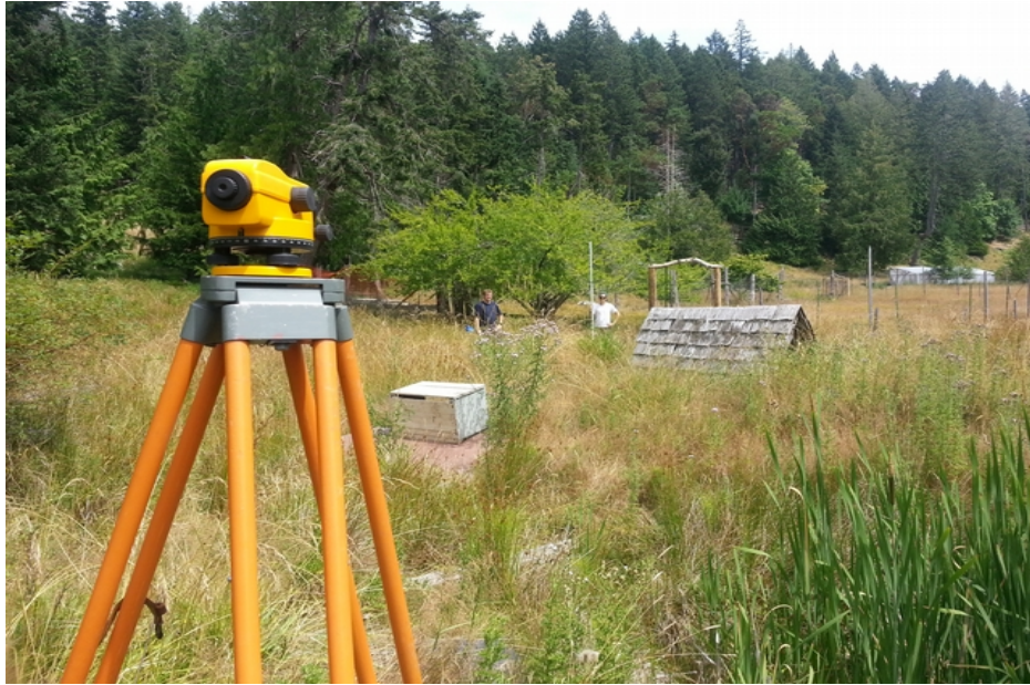
Figure #) Manual surveying using theodolite and rod (determining lowest slope elevation). View from theodolite operator towards meter stick operator.
